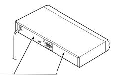
The rating plate and the safety caution are on the rear of the unit.
